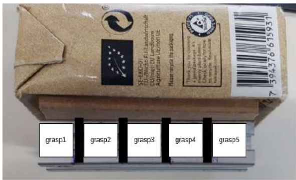
Fig. 7: Validation scenario evaluating the generalizability of ACCIFR across different object grasping positions, representing pose uncertainty during grasping.
