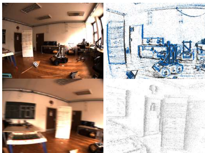
Fig. 3: Sample intensity images and accumulated events (first) and event time surfaces (second) of indoor sequences. In the second sample, motion blur is present in the intensity image, whereas the event time surface remains sharp.
