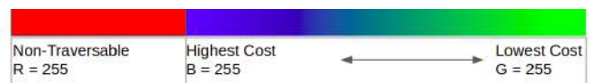
Fig. 3: Cost values are encoded with RGB channels to the terrain point cloud maps.
