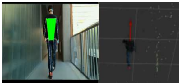
Fig. 3: Detection of pose of a person. The left: the body tracking algorithm and area defined as the torso. On the right, the pose of the person is given by the red arrow with origin at the centroid of the torso of the person.
