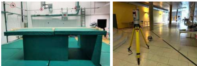
Fig. 5: (Left:) Laboratory test setup in a flycatcher equipped with an Optitrack system. The sphere has IR reflectors attached to its shell, which are detected by the cameras (red circles). (Right:) Laboratory test setup in the Computer Science building. A RIEGL VZ-400 TLS captures a precise ground truth point cloud for comparison with the spherical mobile mapping system. In both images, motion of the sphere is initiated manually by hand.
