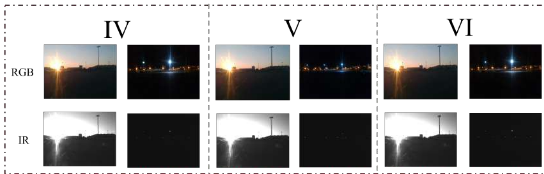
(b) Sun glare versus night. These three pairs of sample images correspond to the peaks in Figure 4(c), where the fusion methods significantly improve the displacement estimation.
