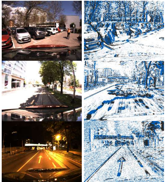
Fig. 1: Sample intensity images (left) and accumulated events (right; color indicates event polarity) from the outdoor sequences. Second sample shows a situation where the left part of the intensity image is overexposed due to bright sunlight as the car is passing through the shaded area, while the event cameras can handle this scenario well, given their high dynamic range. Third sample is captured during a night drive.
