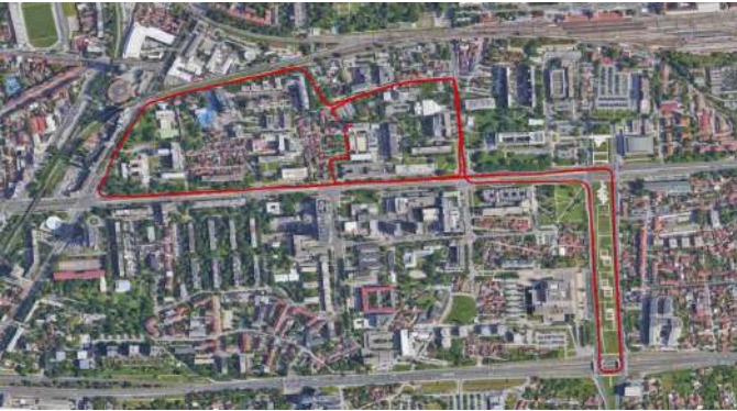
Fig. 4: Ground truth trajectory for a part of our outdoor driving sequences, obtained with a GNSS and AHRS system mounted on the sensor rig placed on the top of the car.
