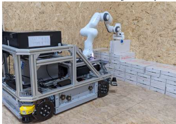
(b) Custom mobile manipulator developed at the Institute for Business Cybernetics for automating the process
