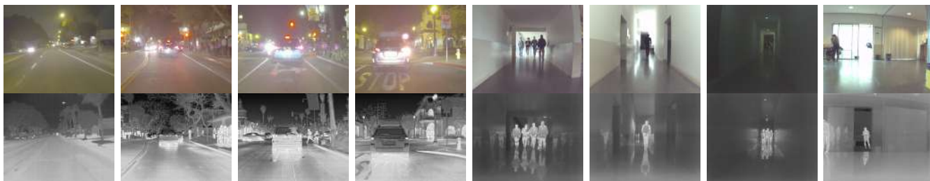
Fig. 2. Selection of scenarios from the FLIR-Aligned dataset [12] (outdoor) and the in-house dataset (indoor) containing RGB and Thermal image pairs, where some limitations of RGB cameras are highlighted. The scenarios contain occlusions, lens flare artifacts, and glow artifacts.
