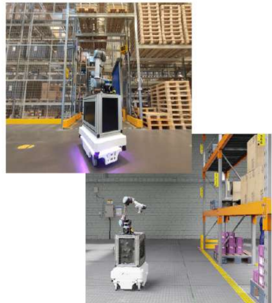
Fig. 1: Typical Novo Nordisk warehouse facility with a custom mobile manipulator (top left), and reference color image of the simulated warehouse facility taken from the WarehouseSIM dataset (bottom right)
