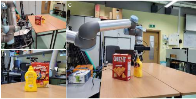
Fig. 9. Experiment with the robot grasping a mustard bottle occluded by the cracker box: initial robot configuration (a,b) and the robot grasping the object (c).
