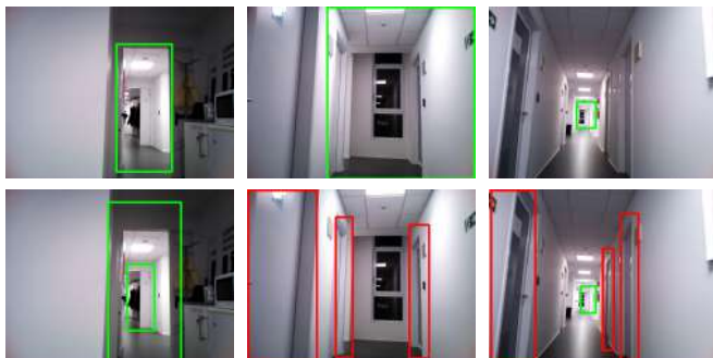
Fig. 9: Challenging nighttime examples classified by GD (top row) and QD_e^{25} (bottom row). QD_e^{25} is fine-tuned with examples obtained with daylight.
