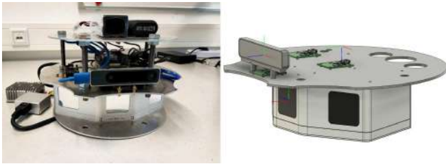
Fig. 3: (Left:) Spherical mobile mapping system without its protecting shell. (Right:) CAD model of the spherical system with sensor frames.
