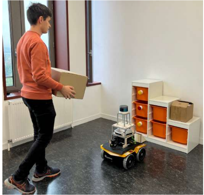
Fig. 1. The experiment to examine the social compatibility of robot navigation. The person works in a room, while the mobile robot moves nearby. The logistic operations at a warehouse are an example of a real scenario, where human workers and autonomous mobile robots need to collaborate with each other and navigate in a shared space.
