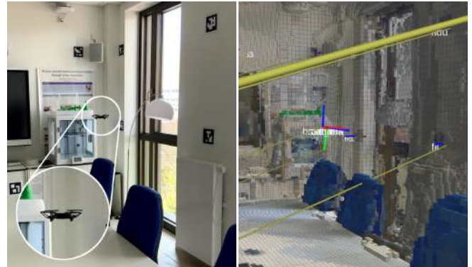
Fig. 1. Comparison of the real environment on the left and the generated 3D occupancy map including the localized fiducial markers and the localized MAV on the right. The left image shows the markers printed on paper and hung up on the walls as well as the MAV. In the right image, the markers can be seen as the darker colored voxels in the occupancy map. The MAV is shown as the coordinate frame in the center of the right image. The yellow rays show the relation between the map origin and frame positions.
