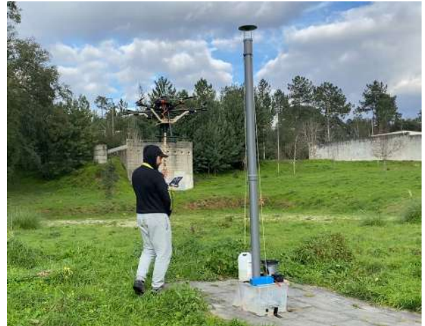
Fig. 2. A field experiment with the human operator. On the left, a human operator guides the Hexa-Copter UAV attached to a vertical pole. On the right, a controllable odour source emits acetone at 3m from the ground.
