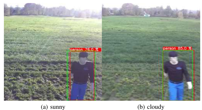
Fig. 1: Example images from the AI-TEST-FIELD with different environment conditions (sunny and cloudy) demonstrating the qualitative differences due to environment conditions. The bounding boxes of the ground truth (green) and the detections of the YOLOv5m trained on the COCO dataset (red) are drawn in the images. Notice that the person here is a dummy and not a real person.
