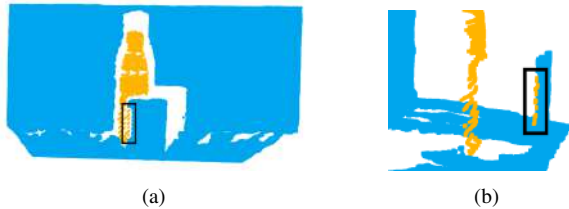
Fig. 7. Instance segmentation errors: (a) general point cloud view, (b) close-up view. If the segmented cloud is not filtered, boundary points on the mask could correspond to other objects. In this case, they correspond to an occluding box.
