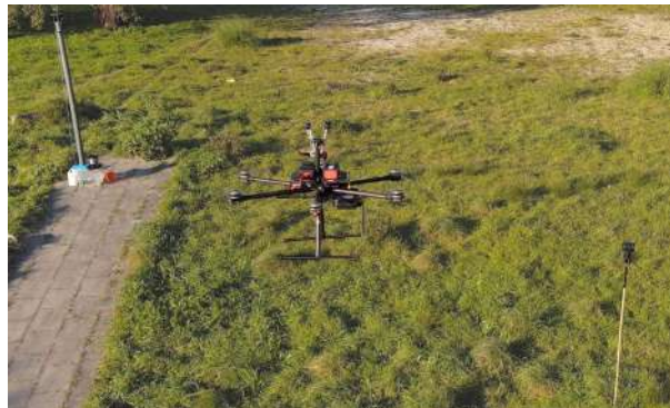
Fig. 1. Testing environment. The image shows the odour source in the left-top corner, a Hexa-Copter UAV in the middle and an ultrasonic anemometer in the right-bottom corner.
