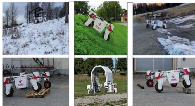
Fig. 1: The figure illustrates the Thorvald II robot’s capability to operate in various rough uneven terrains. To fully utilize the robot’s strengths in these terrains, it is crucial to have a reliable navigation strategy.
