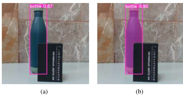
Fig. 2. Object detection methods: (a) bounding box detection, (b) instance segmentation.
