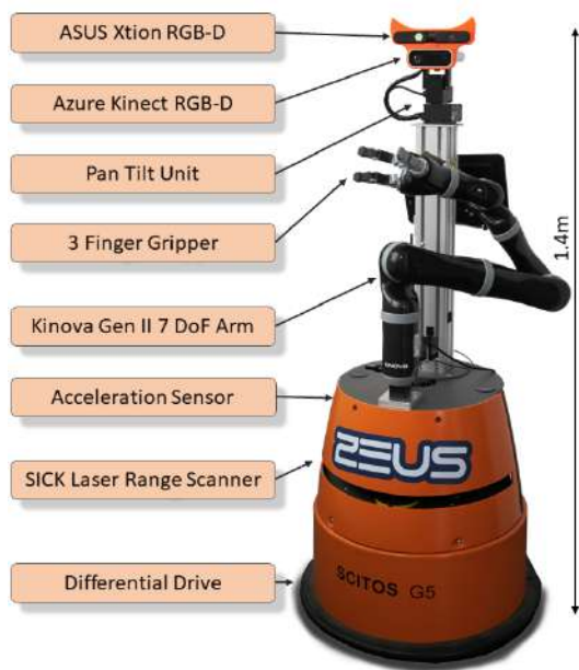
Fig. 1: Robot platform Zeus as a combination of a SCITOS G5 base by MetraLabs GmbH with an arm by Kinova
